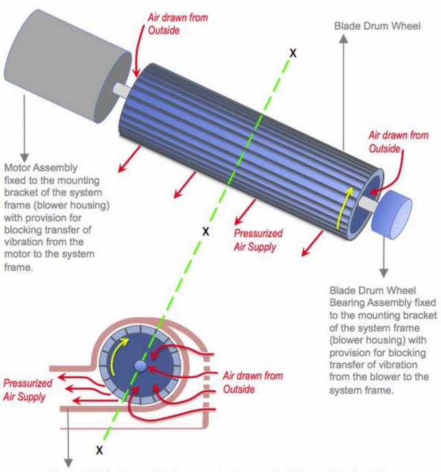
Blower Unit (motor and blade drum wheel assembly) Housing is to be built in part of the system frame directly attached to the air plenum.
